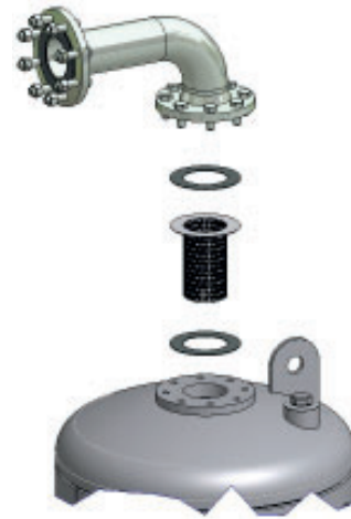
Disassembling of desiccant sieve
