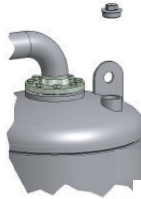
Removing plug from filler sleeve
